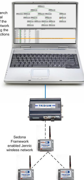
Network Visualization Tool for Sedona Framework enabled Jennic Wireless Networks
